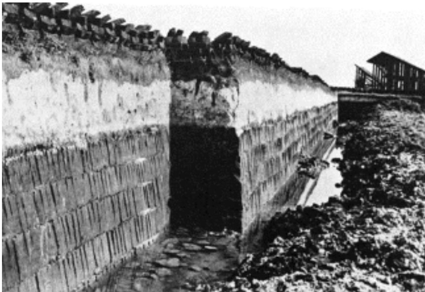
Soil profile from the middle Erdinger Moos. Above the peat lies a layer of about 50 cm thick meadow chalk (Karl Helmut)
