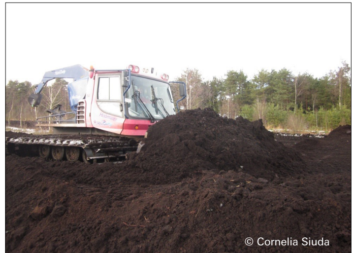
Levelling milled peat fields by a snow ("peat") groomer
