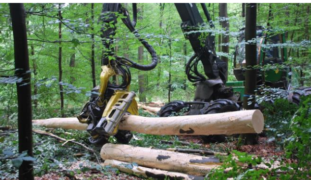
Debarking Head Prototyp (H480C Aggregat John Deere) Foto: IÖL
