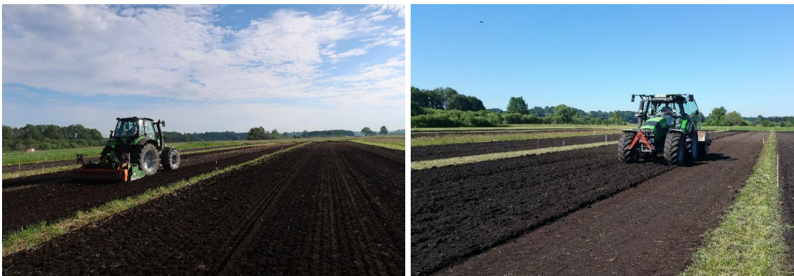
Fig. 2 Left picture: A fine seedbed is created with a rotary harrow. Right picture: Immediately before planting or sowing, the seedbed is compacted with a grassland roller.
