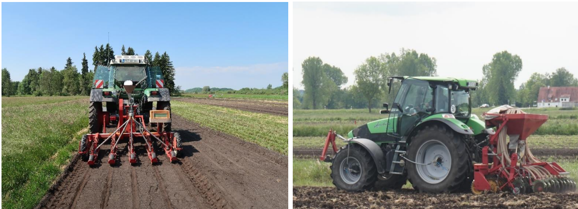
Fig. 3 Left picture: Self-made five-row seed drill machine (manufactured by LfL Landtechnik) for seed rates of < 2 \text{ kg ha}^{-1} . Right picture: Universal drill seeder during the seeding of reed canary grass at the study site Riedhausen.
